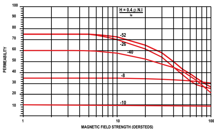
Incremental permeability \mu versus D.C magnetizing force
